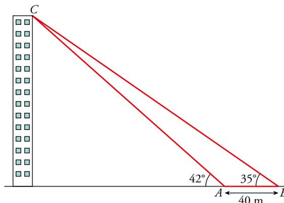
$$\left. \begin{aligned} \operatorname{tg} 42^\circ &= \frac{h}{d} \rightarrow h = d \operatorname{tg} 42^\circ \\ \operatorname{tg} 35^\circ &= \frac{h}{d+40} \rightarrow h = (d+40) \operatorname{tg} 35^\circ \end{aligned} \right\} \rightarrow$$
